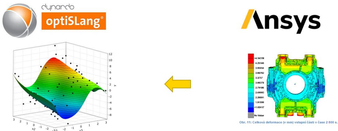
Figure 2. Procedure for creating a metamodel for a digital twin using Ansys software
